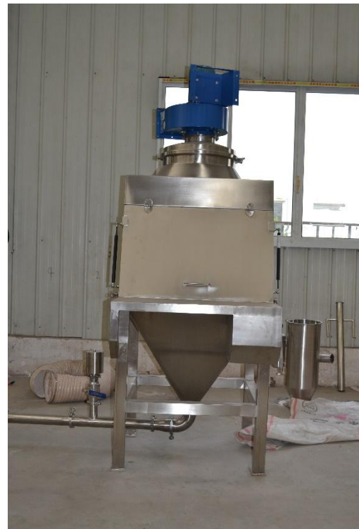
Rip and Tip Unloading Station with filter.
